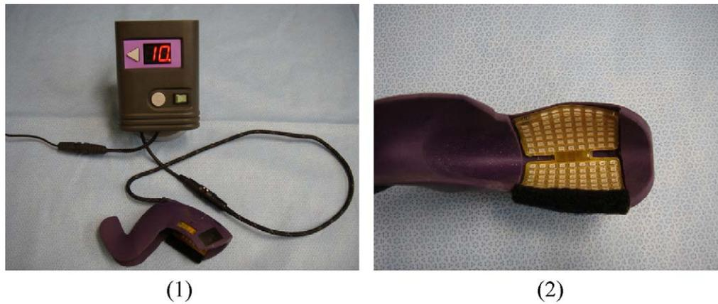
**Fig. 2.** (1) The light therapy device. Once the button is pressed, the LED irradiation begins and continues for 10 min. (2) The LEDs are mounted to the underside of the custom-designed brace, the brace is fitted on the knee joint, and then wrapped with bandaging.
